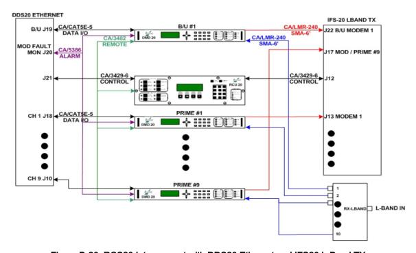
Figure B-20. RCS20 Interconnect with DDS20 Ethernet and IFS20 L-Band TX
