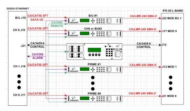
Figure B-33. RCS20 Interconnect with DDS20-GIGE-M and IFS20 L-Band
