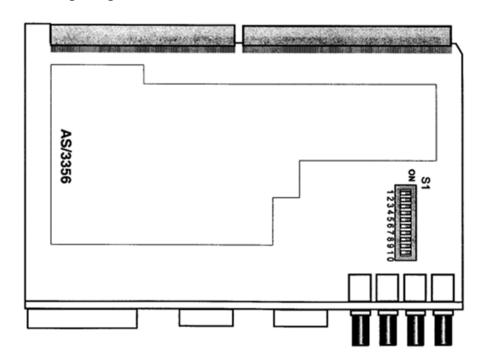
Figure 5-9 AS/3356 Data Switch Module
