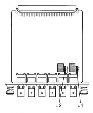
Figure 5-4 Reference Distribution Module Jumper Settings
