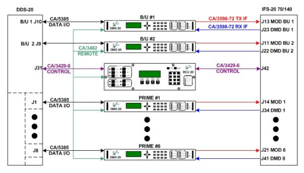
Figure B-4. RCS20 interconnect with DDS20 and IFS-20 70/140
