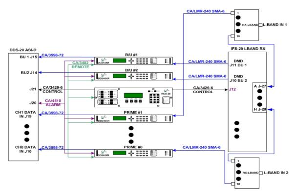
Figure B-31. RCS20 Interconnect with DDS20-ASI-M and IFS20 L-Band TX
