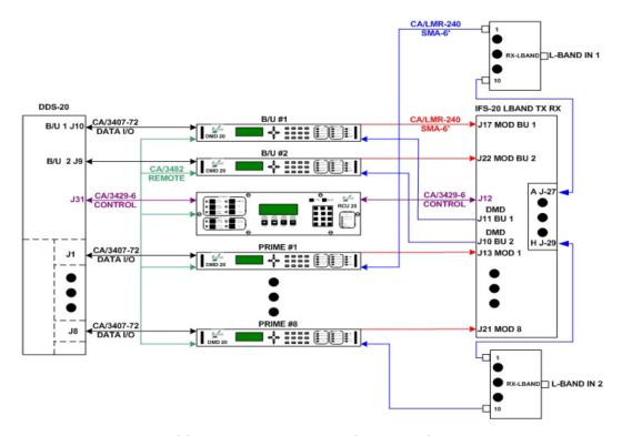
Figure B-10. RCS20 Interconnect with DDS20 and IFS20 L-Band TX/RX
