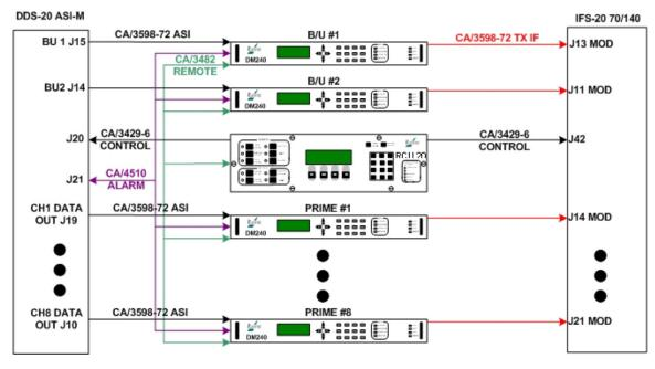
Figure B-25. RCS20 Interconnect with DDS20-ASI-M and IFS20 70/140
