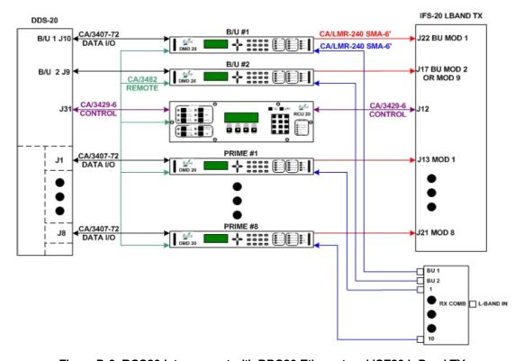
Figure B-6. RCS20 Interconnect with DDS20 Ethernet and ISF20 L-Band TX
