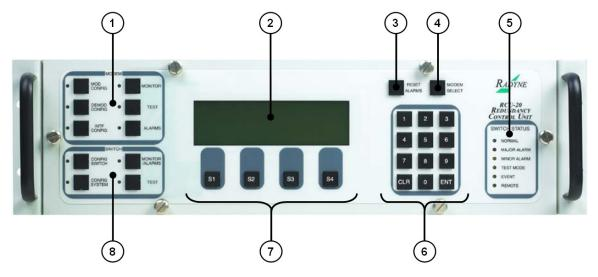
Figure 4-1. Front Panel Interface
