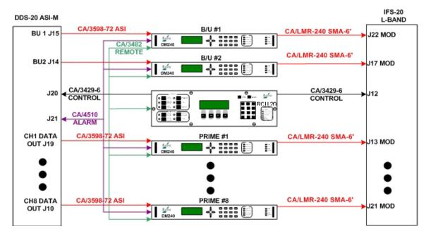
Figure B-27. RCS20 Interconnect with DDS20-ASI-M and IFS20 L-Band
