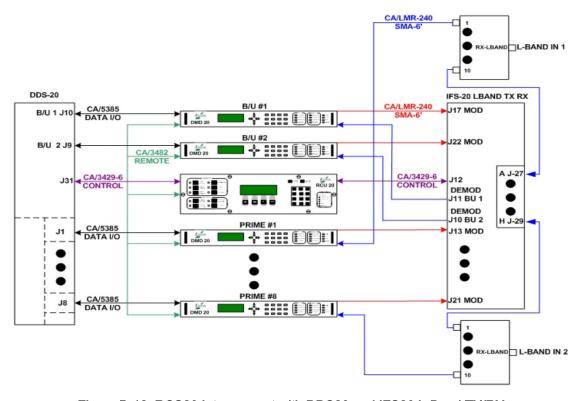
Figure B-12. RCS20 Interconnect with DDS20 and IFS20 L-Band TX/RX
