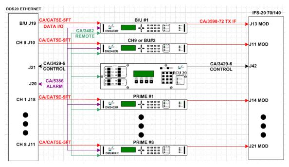
Figure B-35. RCS20 Interconnect with DDS20-GIGE-M and IFS20 70/140
