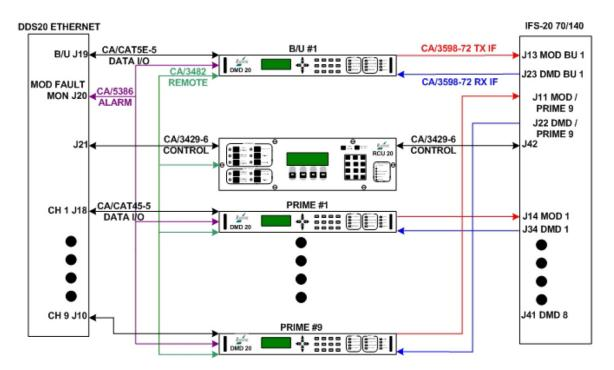
Figure B-18. RCS20 Interconnect with DDS20 Ethernet and IFS20 70/140
