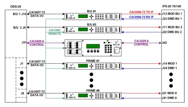
Figure B-2. RCS20 interconnect with DDS20 and IFS-20 70/140
